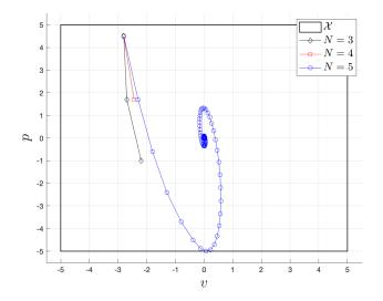
The MPC problem is not feasible at time step t = 3 when N = 3. The MPC problem is not feasible at time step t = 1 when N = 4.
