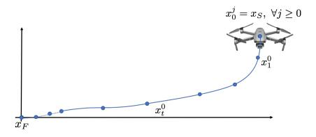
Iteratively drive the drone to a goal state  $x_F$  from an initial state  $x_S$ .
