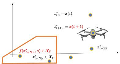
Notice that  $J_t^*(x_t) = \sum_{k=t}^{t+N-1} h(x_{k|t}^*, u_{k,t}^*) + V(x_{t+N|t}^*) \ge h(x_{t|t}^*, u_{t,t}^*) + \sum_{k=t+1}^{t+N-1} h(x_{k|t}^*, u_{k,t}^*) + h(x_{t+N|t}^*, u) + V(f(x_{t+N|t}^*, u))$
