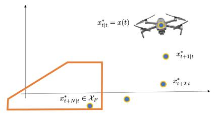
Let  $\{x^*_{t|t}, \dots, x^*_{t+N|t}\}$  and  $\{u^*_{t|t}, \dots, u^*_{t+N-1|t}\}$  be the optimal state-input sequences.
