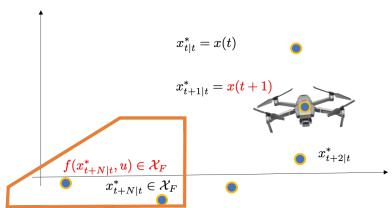
At t + 1, the state sequence  $\{x_{t+1|t}^*, \dots, x_{t+N|t}^*, f(x_{t+N|t}^*, u)\}$  and input sequence  $\{u_{t+1|t}^*, \dots, u_{t+N-1|t}^*, u\}$  are feasible.
