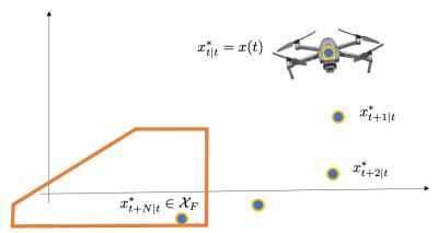
Let  $\{x^*_{t|t},\ldots,x^*_{t+N|t}\}$  and  $\{u^*_{t|t},\ldots,u^*_{t+N-1|t}\}$  be the optimal state-input sequences.
