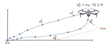
Iteratively drive the drone to a goal state  $x_F$  from an initial state  $x_S$ .
