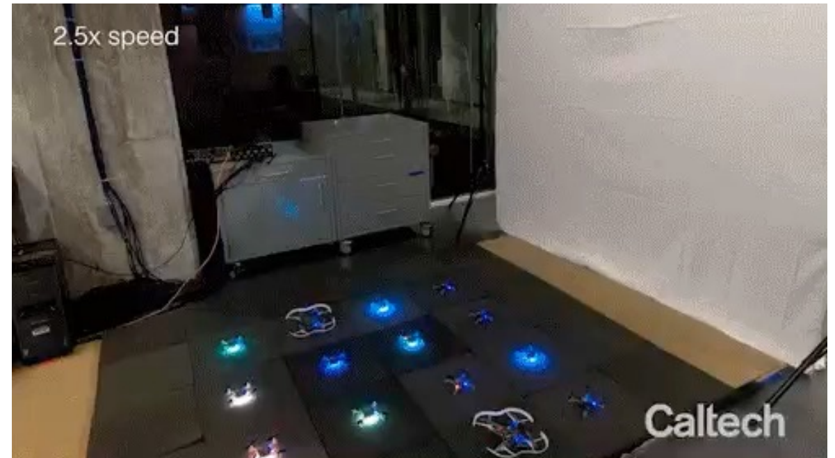
16-robot 3-ring tracking task (2 large, 14 small)
